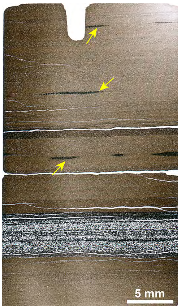
Fig. 15 Detail view of the lowermost Genesee. It is a black shale with well-developed pyritic streaks (yellow arrows) that occur in three discrete horizons and very much resemble those seen in the New Albany (Fig. 5) and Bakken shales
