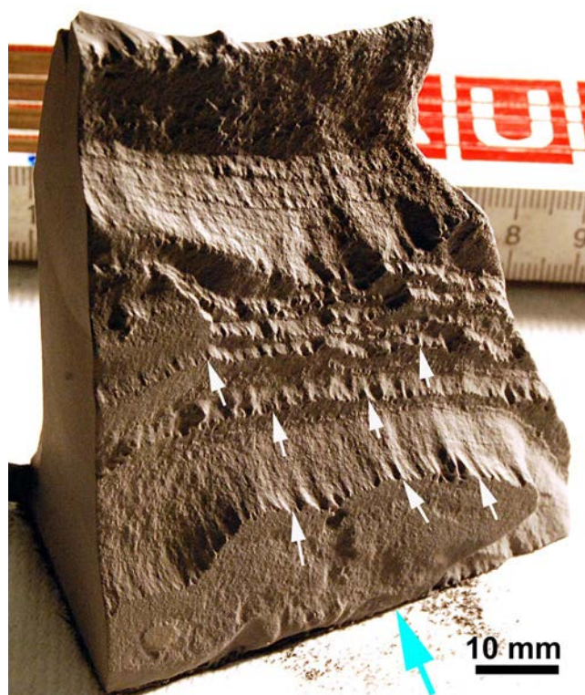
FIGURE 7 Another sample of shale (New Albany Shale, Indiana) with alternating silt (harder) and mudstone layers (softer). Layering is vertical. White arrows point to flute development in mudstone layers, downwind (blue arrows = airflow direction) of resistant siltstone layers
