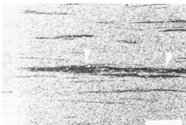
Fig. 15. Carbonaceous flakes in dolomitic clayey shale. Note that silt grains are associated with and included in carbonaceous flakes. Lamination in the large fragment in the centre has internal laminae (arrows) that are the same as in beds of carbonaceous silty shale. Scale bar is 0.5 mm long.
