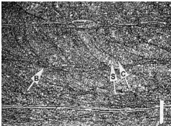
Figure 9: Photomicrograph of micro-laminated silty mudstone (BM-1), showing alternating micro-cross-laminae of silt (arrow S) and clay (arrow C) within macroscopically visible laminae (arrow I points out macroscopic lamina boundaries). These micro-cross-laminae are probably compacted Zoophycos back-fill menisci. Compare with Figure 7A. Scale bar is 1 mm long.
