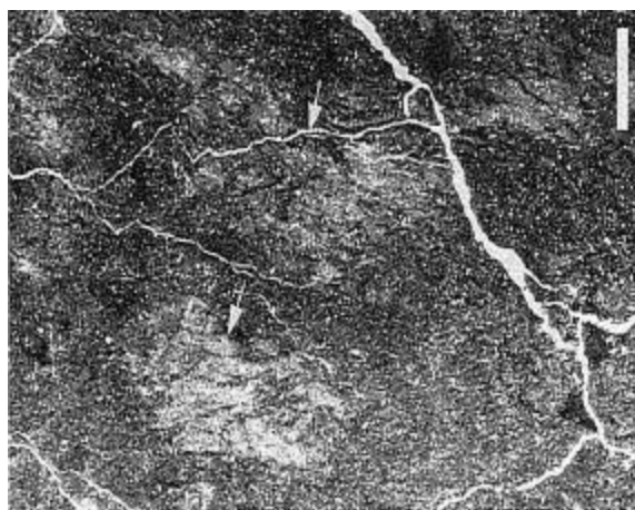
Figure 5: Photomicrograph of mottled red mudstone (RM-2), shows mottled texture. Bleached, light-colored cloudy areas (arrows) are probably developed along small root traces. Compare with Figure 3B. Scale bar is 2 mm long.
