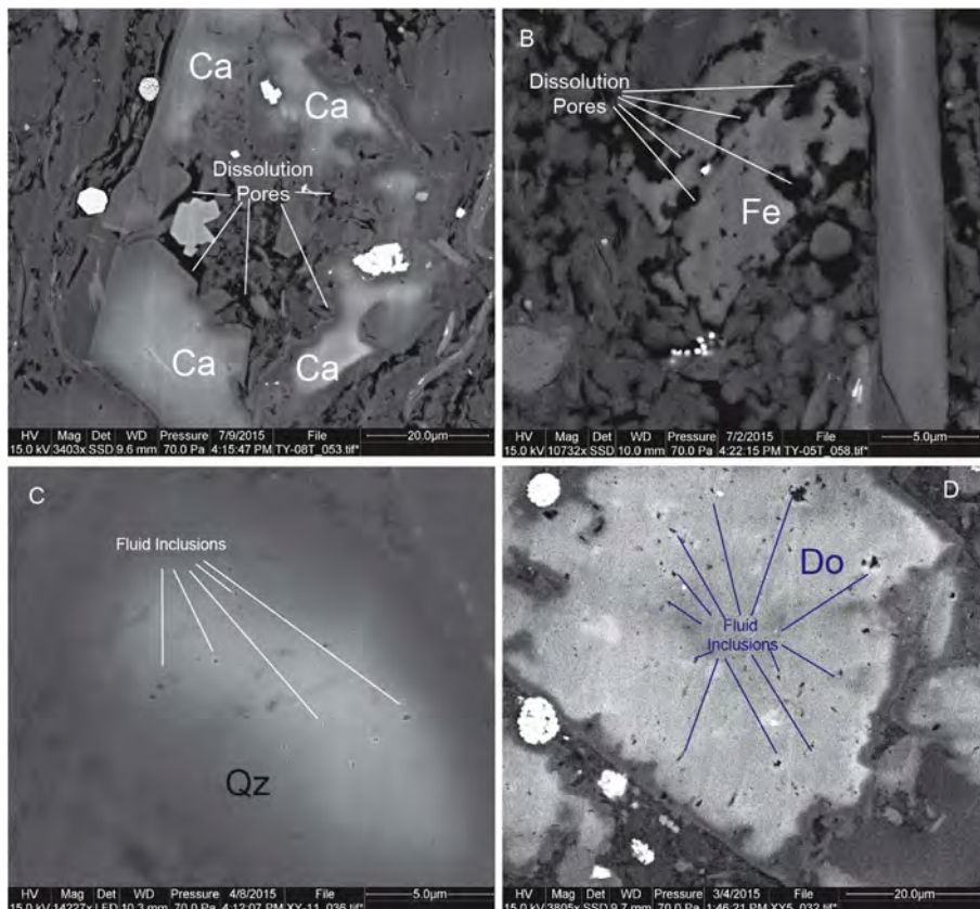
Fig. 8. Characteristics of dissolution pores and Fluid inclusions. (A) Dissolution pores within calcite (BSE image), Longmaxi Formation, Well Xiye-1; (B) Dissolution pores within feldspar (BSE image), Wufeng Formation, Well Tongye-1; (C) Fluid inclusions within quartz (SE image), Longmaxi Formation, Well Xiye-1; (D) Fluid inclusions within dolomite, Guanyinqiao Formation, Well Tongye-1. Ca = calcite; Do = dolomite; Qz = quartz; Fe = feldspar. All the surfaces in SEM images are perpendicular to bedding. In these images bedding is oriented vertical.
