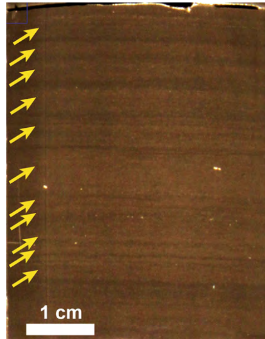
Fig. 17 Compositional banding in a piece of drill core from the Middle Devonian Geneseo Shale. Yellow arrows point to compositional bands with fuzzy-gradational boundaries
