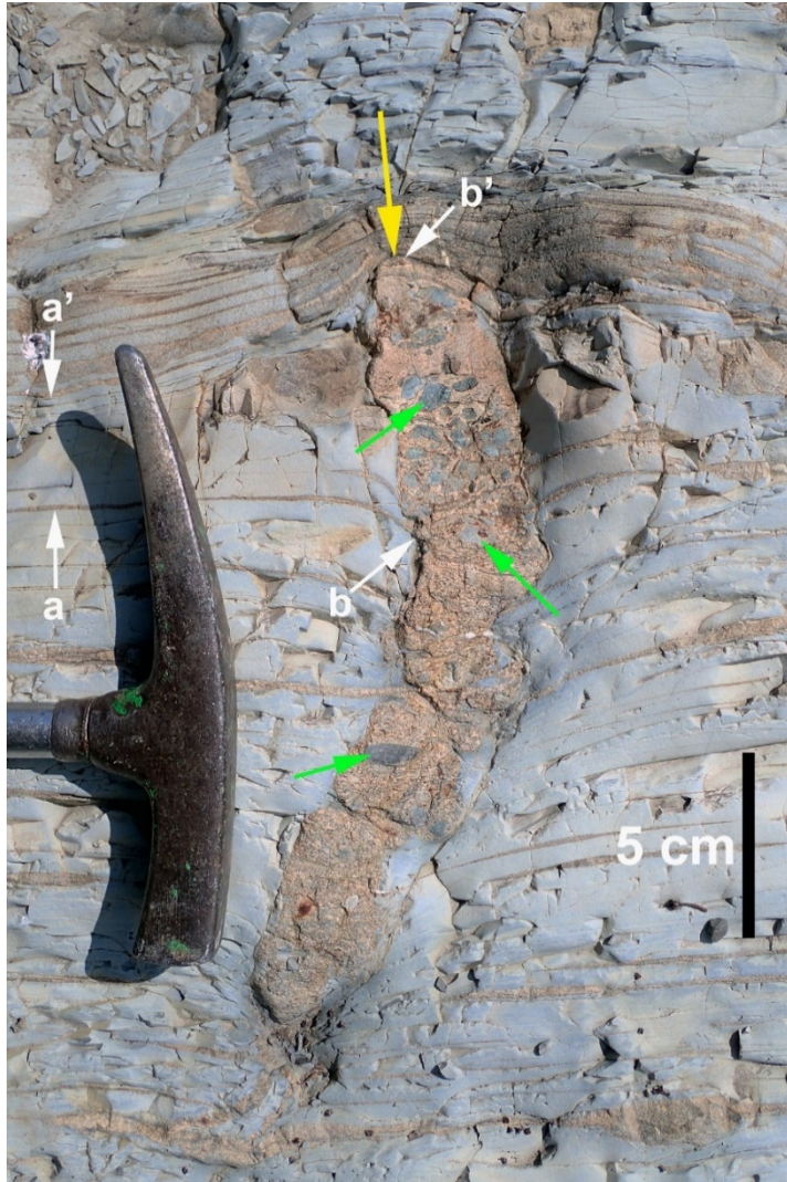
Figure B: A fissure filled with sand and green pebbles (metamorphic, green arrows). The infilling sediment is not of the same composition than that of the sand layer that drapes over the top (yellow arrow). Differential compaction for sediment horizons marked by arrows a-b and a'-b' suggests that the sediment contained about 60 vol % water when the fissure was filled.
